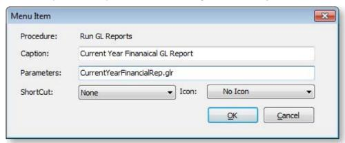
Specifying a .GLR file means that when the menu item is selected, a GL report will be automatically generated using the settings in the .GLR file (the Run GL Report window does not appear). It is possible to set up multiple GL Report menu items, each with different settings, so that a variety of GL Reports can be generated quickly.
